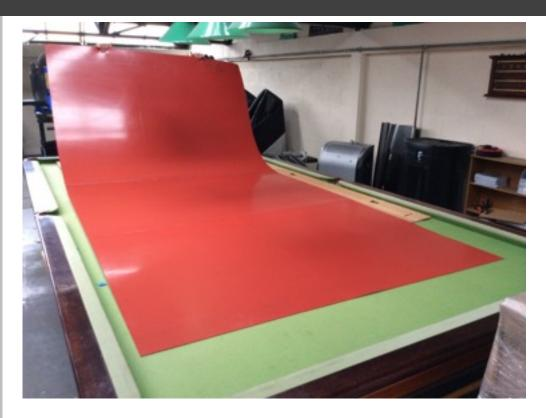
LaminaHeat **PowerBlanket** Heaters are used in the composite industry to bond and cure composite structures using state of the art processing technologies like vacuum bagging techniques, upgrading cold presses to heated presses or heating metal moulds for a variety of processing industries.
